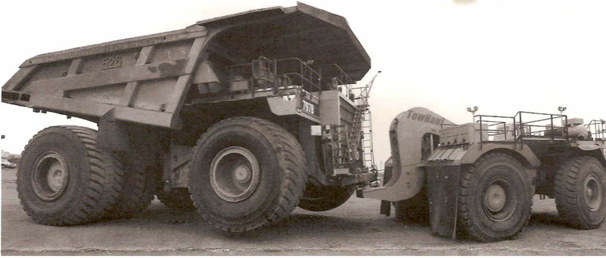
Two retired 793 heavy haulers were converted into rescue vehicles to pull disabled haulers out of the mines. photo by Bob Nyen
